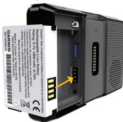
Installing the Battery
