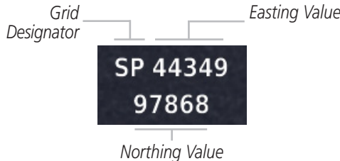
Figure 16-44 British National Grid Position Format Detail
