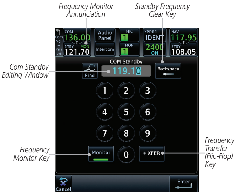
Figure 3-24 Com Frequency Monitoring
