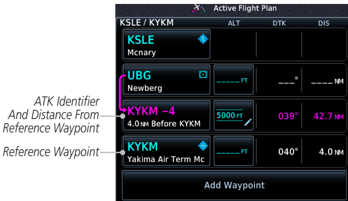
Figure 4-13 ATK Inserted Before Reference Waypoint
