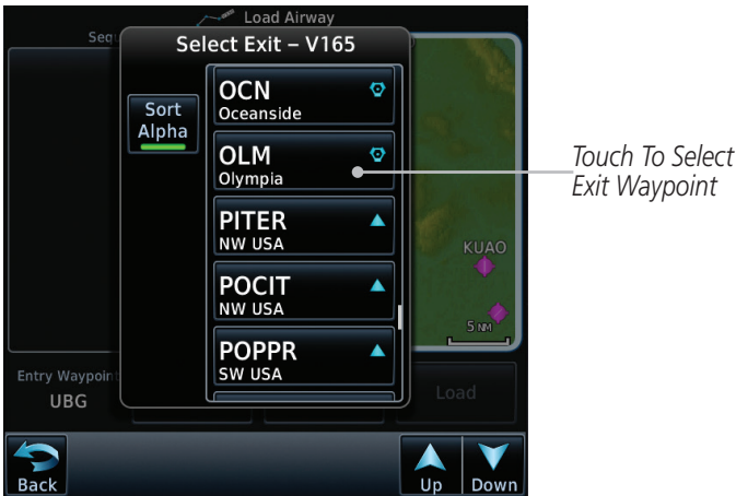
Figure 4-23 Select an Exit Waypoint for the Airway
