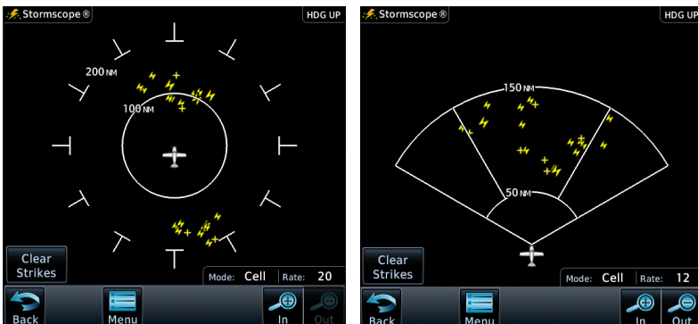
Figure 12-49 StormScope 360° and Arc Display Views
