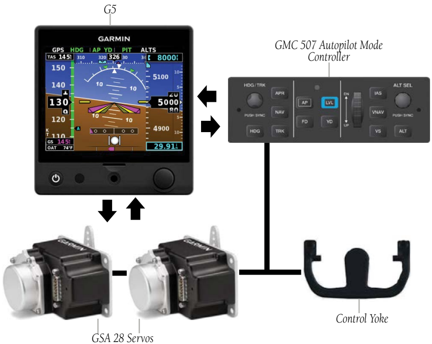
Figure 3-1 Core GFC 500 System
