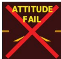
Figure 1-6 Attitude Failure Indication
