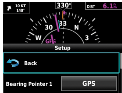
Figure 2-20 Bearing Pointer Setting
