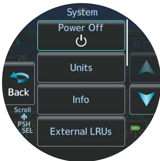
Battery Power-Off Menu
