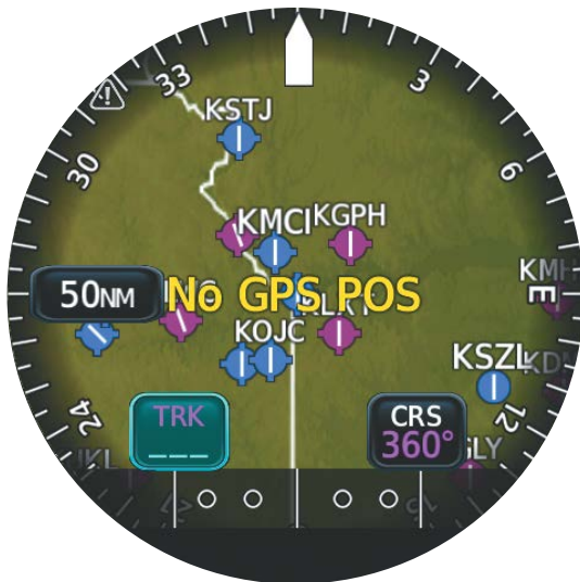
Complete Loss of GPS - 'No GPS POS' annunciation on 'HSI Map' Page
