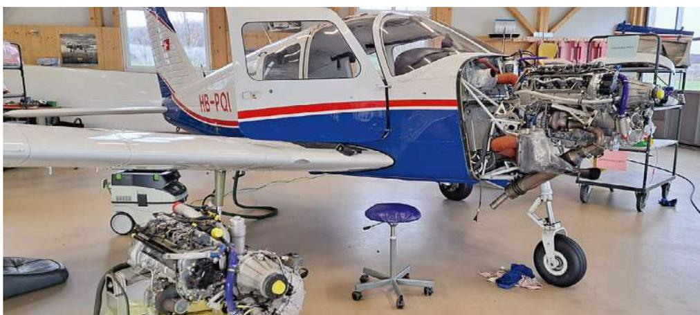
Links: Motorenwechsel in der Maintenance Birrfeld.
